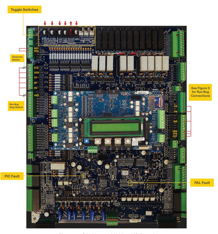
Figure 4: GALX-1102AN Main I/O Board
